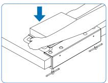
The build platform jig is designed to stabilize the build platform for the secure removal of prints. Secure the build platform jig to the edge of your work surface by tightening the jig screw clamps underneath the work surface. The build platform jig can also be secured to the work surface using the two screw holes on the front of the jig. Ensure that there is enough space in front of the jig for the build platform.
