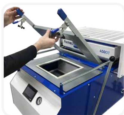
5. Then locate it at the front of the clamp frame. The hole on the top plate of the reducing window needs to be at the front of the machine.
