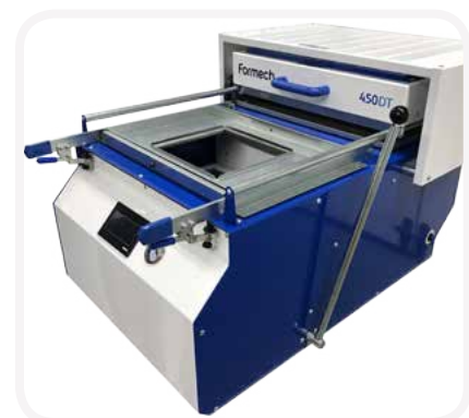
6. Close and lock the clamp frame. At this stage, you may have to adjust the toggle clamps.
