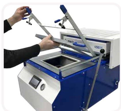
4. Place the upper reducing window in the clamp frame at the rear.
