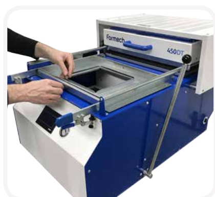
7. Fit the bolt and the nut to secure the window to the clamp frame.
