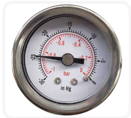
A vacuum gauge reading of 22”Hg or higher is normal. A lower reading indicates poor vacuum where attention is required
