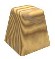
Add draught angle/radius corners to allow the material to flow over the tool/mould/pattern.
