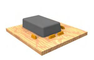
Place angled blocks around the corners to use up the excess material.
