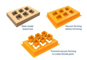
This method of using a male tool to produce female formings can be used for reel feed material where a female or negative vacuum forming (position below the clamp) would cause problems when trying to advance the formed sheet through the machine, unless your machine features a negative gate.
