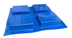
Multiple tooling can create une-qual material stretching on the sides.
